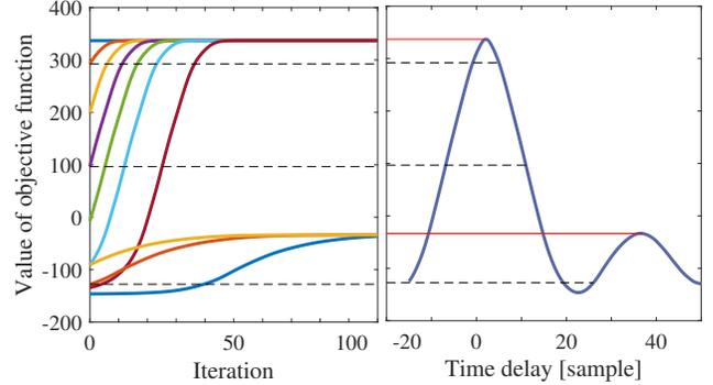
Figure 1: Left: the value of objective function via the proposed method over initial values. Different curves represent different values of the initial time delay estimate, taken every 3 samples from 2 to 29. Right: objective function.
