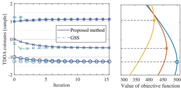
Figure 2: Left: TDOA estimates in the reverberant environment with the SNR of 10 dB;  $\circ$ , DOA is  $30^\circ$ ;  $\times$ , DOA is  $70^\circ$ ;  $*$ , DOA is  $135^\circ$ . Right: value of the objective function corresponding to respective DOAs.
